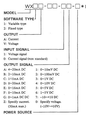
Ordering Information Measuring Range of Input Voltage input signal: 2V min. Span for 0~10V DC Current input signal (input resist.  $250\Omega$ ):  $(250\Omega) \times (Input current)$  shall be within the measuring span of voltage input signal. Recommended Range 4~20mA DC 2~10mA DC Current signal 0~20mA DC 0~16mA DC 0~10mA DC 0~10V DC Voltage signal 0~ 5V DC 1~ 5V DC
